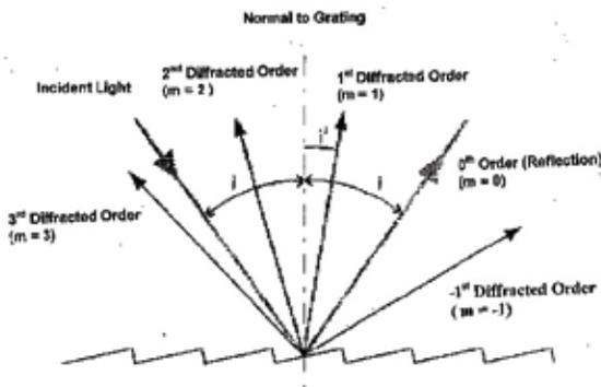
A diffraction grating is an optical component with a regular pattern of elements or grooves. All gratings have intensity maxima at angles  $\theta_m$  which are given by the grating equation
