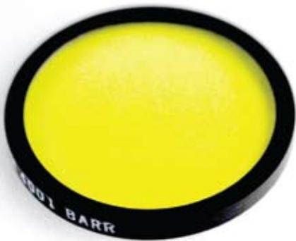
Suppression of higher diffraction orders in a grating-based instrument is often achieved by use of an Order Sorting Filter comprised of a longpass or bandpass filter coating on a thin glass substrate. The blocking band of the interference filter coating affords rejection of undesired diffraction orders.
