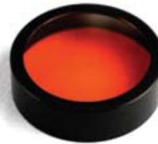
Barr can provide simple absorption-glass-type filters for order sorting. Filters of this type are constructed using color filter glass selected to provide transmission over the wavelength range required for sensing of the desired diffractive order while attenuating (by absorption) the shorter wavelengths associated with higher diffraction orders.
