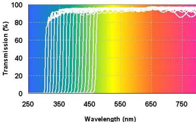
Barr designs and manufactures both edge-type and bandpass-type LVF's to customer specifications, and both types of LVF's are sometimes used as Order Sorting Filters in grating-based systems. For example, a Linear Variable Filter can be used in an imaging spectrograph to provide order sorting when used with a focal plane detector.
